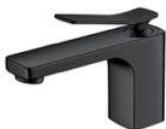
Model: 1095B (Brass) Single-lever basin mixer Height: 142mm, spout projection: 138mm Ceramic cartridge: 35mm Finished: Matte Black
