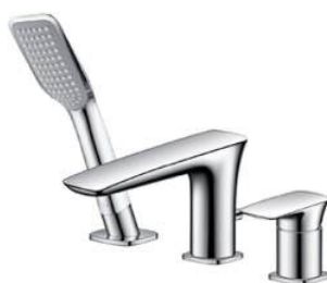
Model: 6198 (S077) 3-piece bath-shower mixer Height: 130mm, spout projection: 200mm Ceramic cartridge: 40mm Hand shower: S082W, ABS, 1-function Hose: 150mm Finished: Chrome
