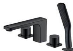
Model: 6295B (S082B) 4-piece bath-shower mixer Hand shower: S082W, ABS, 1-function Hose: 150mm Ceramic cartridge: G1/2mm Finished: Matte Black
