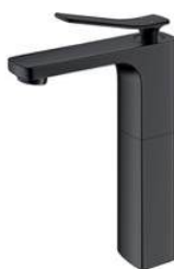
Model: 1295B (Brass) Single-lever basin mixer Height: 290mm, spout projection: 138mm Ceramic cartridge: 35mm Finished: Matte Black
