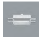
82922.000 Mounting frame For flush mounting of luminaires with ceiling aperture 168x168mm. Polymer, white (RAL9002). Mounting for ceiling thicknesses of 12.5-25mm. The recess depth of the luminaire increases by 2mm. Weight 0.2kg
