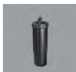
34974.000 Distribution box, IP68 With four cable entries, 7-25mm. Polymer. ø 102mm, L 305mm. Weight 0.47kg
