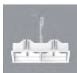
83968.000 Mounting frame, 2x Polymer, white (RAL9002). Mounting without tools for ceiling thicknesses up to 30mm. Covered mounting detail. Recess depth: 260mm for directional luminaires and 220mm for downlights and recessed spotlights. Weight 0.3kg
