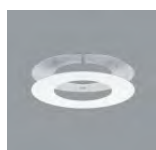
88290.000 Compensation set For over-large ceiling aperture. Lock ring: steel sheet, galvanised. Mounting for ceiling thicknesses of 15-25mm. Cover ring: metal, white. When ordering state ceiling aperture of the luminaire and diameter of the available ceiling aperture.
