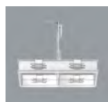
83969.000 Mounting frame, 2x Polymer, white (RAL9002). Mounting for ceiling thicknesses of 12.5-25mm. Flush mounting detail. Recess depth: 260mm for directional luminaires and 220mm for downlights and recessed spotlights. Weight 0.3kg
