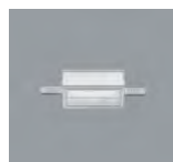
82921.000 Mounting frame For flush mounting of luminaires with ceiling aperture 133x133mm. Polymer, white (RAL9002). Mounting for ceiling thicknesses of 12.5-25mm. The recess depth of the luminaire increases by 2mm. Weight 0.15kg
