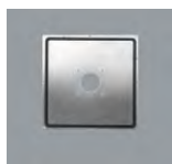
83598.000 Spacer plate Aluminium. For flush-mounting of downlights in concrete housings in exposed concrete ceilings. Weight 0.05kg
