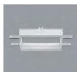
82923.000 Mounting frame For flush mounting of luminaires with ceiling aperture 206x206mm. Polymer, white (RAL9002). Mounting for ceiling thicknesses of 12.5-25mm. The recess depth of the luminaire increases by 2mm. Weight 0.3kg
