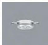
82936.000 Mounting ring For flush mounting of luminaires with ceiling aperture Ø 131mm. Polymer, white (RAL9002). Mounting for ceiling thicknesses of 12.5-25mm. The recess depth of the luminaire increases by 2mm. Weight 0.1kg
