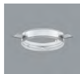
82938.000 Mounting ring For flush mounting of luminaires with ceiling aperture Ø 206mm. Polymer, white (RAL9002). Mounting for ceiling thicknesses of 12.5-25mm. The recess depth of the luminaire increases by 2mm. Weight 0.2kg
