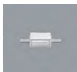
82920.000 Mounting frame For flush mounting of luminaires with ceiling aperture 104x104mm. Polymer, white (RAL9002). Mounting for ceiling thicknesses of 12.5-25mm. The recess depth of the luminaire increases by 2mm. Weight 0.15kg
