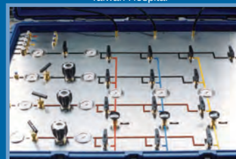
Job 419 Year 1996 3 Diver Gas Panel for Taiwan Navy
