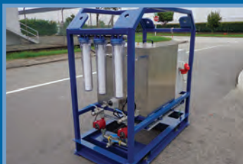
Job 1340 Year 2012 Chemical Flushing Unit
