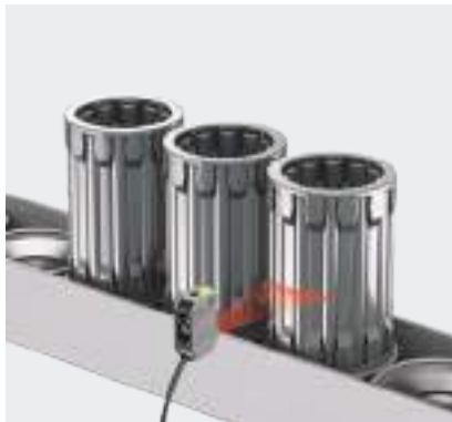
Presence detection of needle bearings
