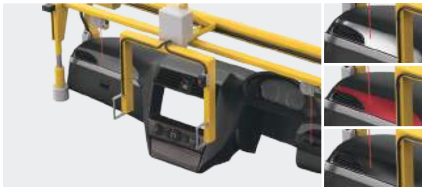
Presence detection of interior decoration parts
