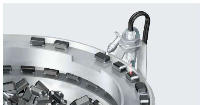
Air blower output during chip's front/rear detection
