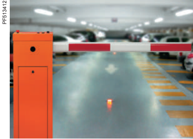
ATV12 controlling an access barrier
