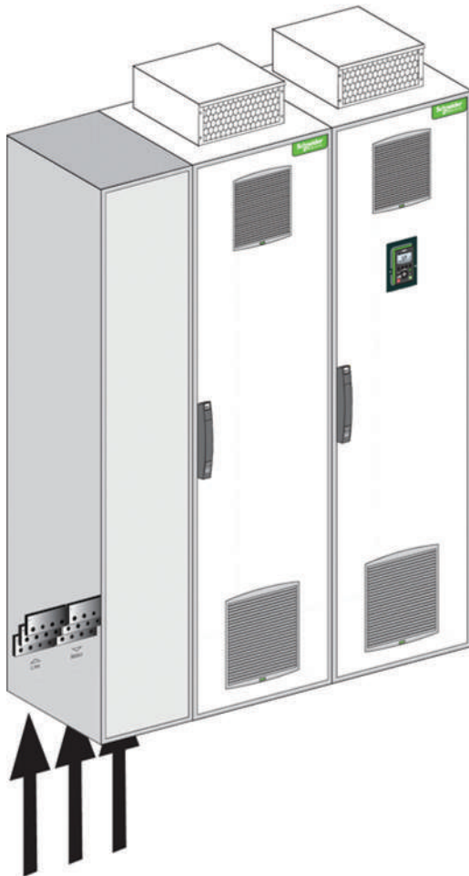
Additional enclosure allowing cabling from the bottom
